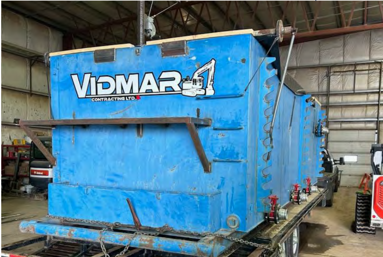
Figure 8: Settling tank in shop. Drain valves shown
