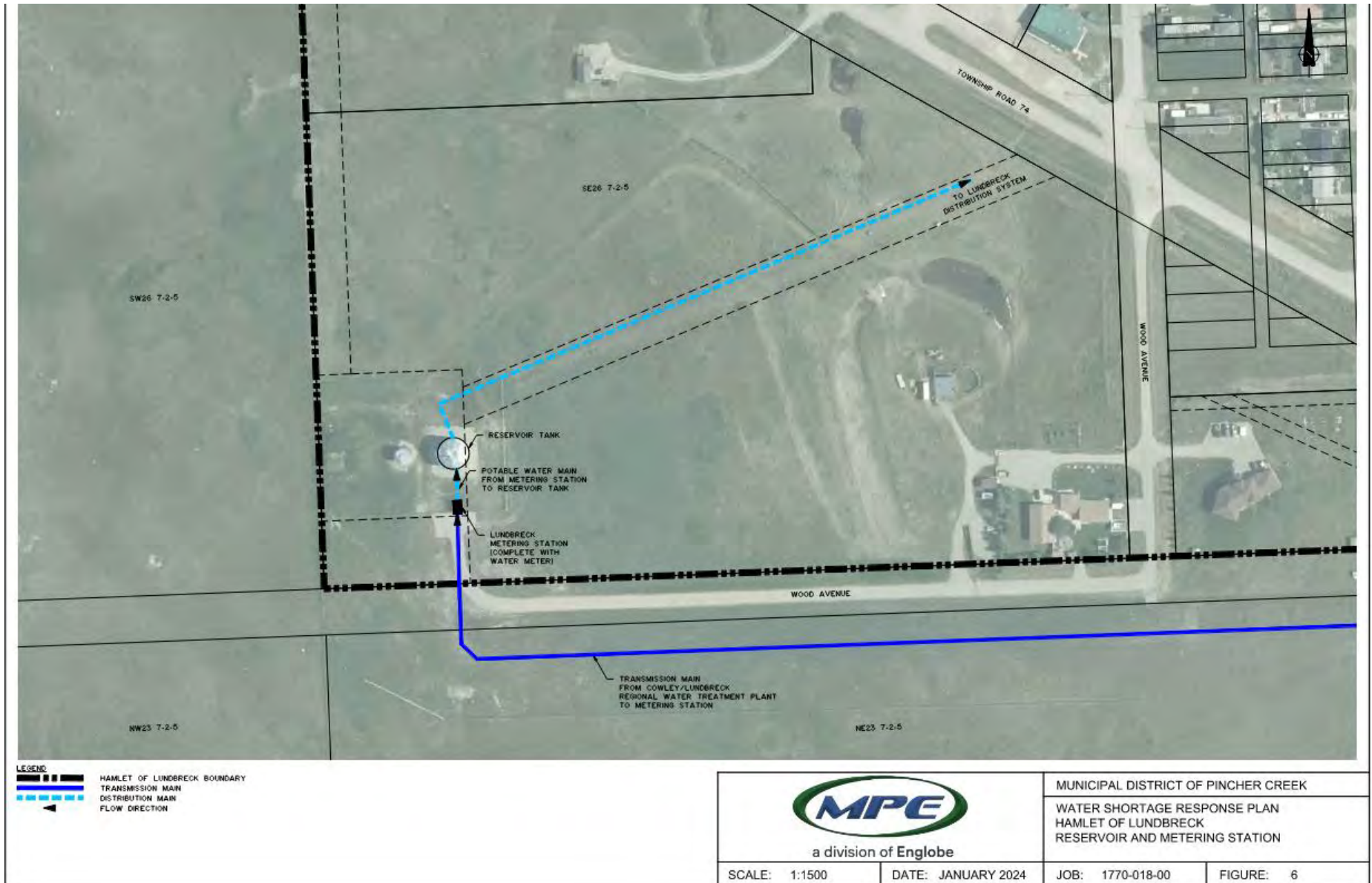
FIGURE 14: HAMLET OF LUNDBRECK CONNECTION & RESERVOIR
