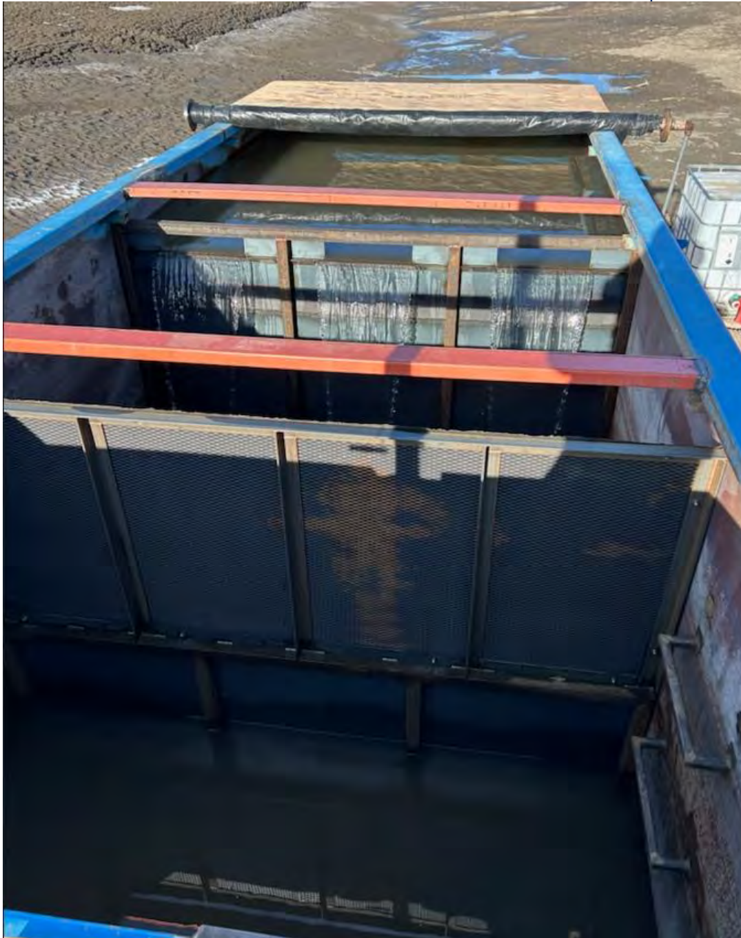
Figure 7: Settling tank top view while filling. Requires additional pump (not shown) and nightly emptying
